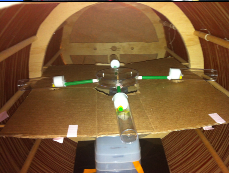
Interior view of the solenoid design and placement of choice chamber
