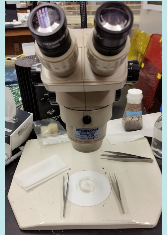
Figure 2. Microdissection setup with forceps and dissection plate under a dissecting microscope.
