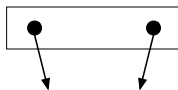
Figure 15.2: For an extremely large elevator, and over extreme distances, two balls in a box approach each other – evidently, to distinguish between constant acceleration and gravity one needs to compare two falling objects.
